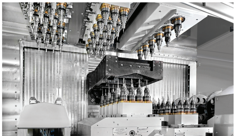
HCX transfer centers from ANGER MACHINING invert the logic of traditional machining centers: It is not the spindle that moves to the part. Instead, the part – mounted on a movable clamping fixture (black, center) – is moved against the spindles that are mounted on the machine's frame in part-specific groups.
