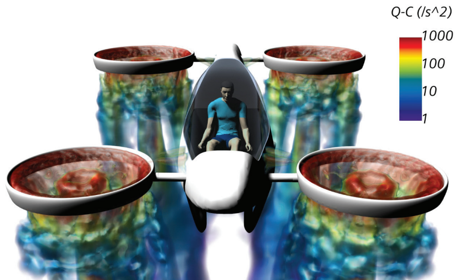
Figure 4. Visualization of the prop wash from an urban air mobility vehicle where the propeller effects were computed using the blade element method.
